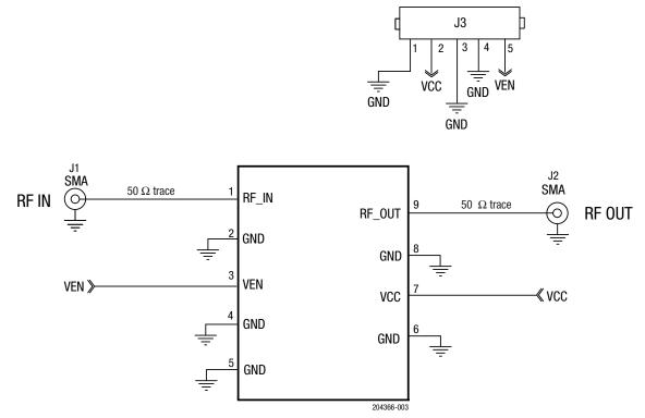
Figure 3. SKY65725-81 Evaluation Board Schematic
