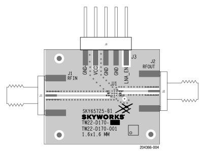
Figure 4. SKY65725-81 Evaluation Board Assembly Diagram
