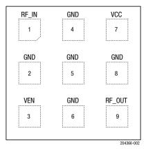
Figure 1. SKY65725-81 Pinout (Top View)
