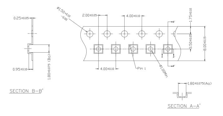
10 SPROCKET HOLE PITCH CUMULATIVE TOLERANCE :  $\pm 0.20\,\text{mm}$  Ao & Bo MEASURED ON PLANE 0.30mm ABOVE THE BOTTOM OF THE POCKET. ALL DIMENSIONS ARE IN MILLIMETERS.
