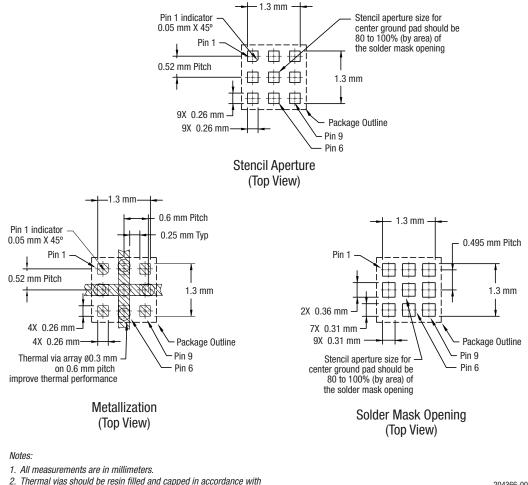
πιστιται vias should be resimined and capped in accordance with IPC-4761 type VII vias. Recommended Cu thickness is 30 to 35 μm. 204366-005
