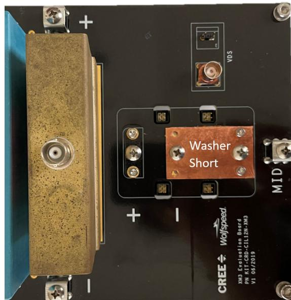
**Figure 2.2. Low-Side Short Circuit Setup with Large Copper Bus Bar**
