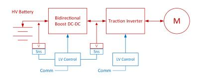
HEVs also include a generator that converts mechanical energy from the internal combustion engine (ICE) into electrical energy to recharge the battery when the ICE is running. A block diagram for the generator's ac-dc converter looks the same as the traction inverter, with the motor ("M") replaced with a generator and the power flowing from generator towards the HV battery. Isolated gate drivers are needed for the switches.
