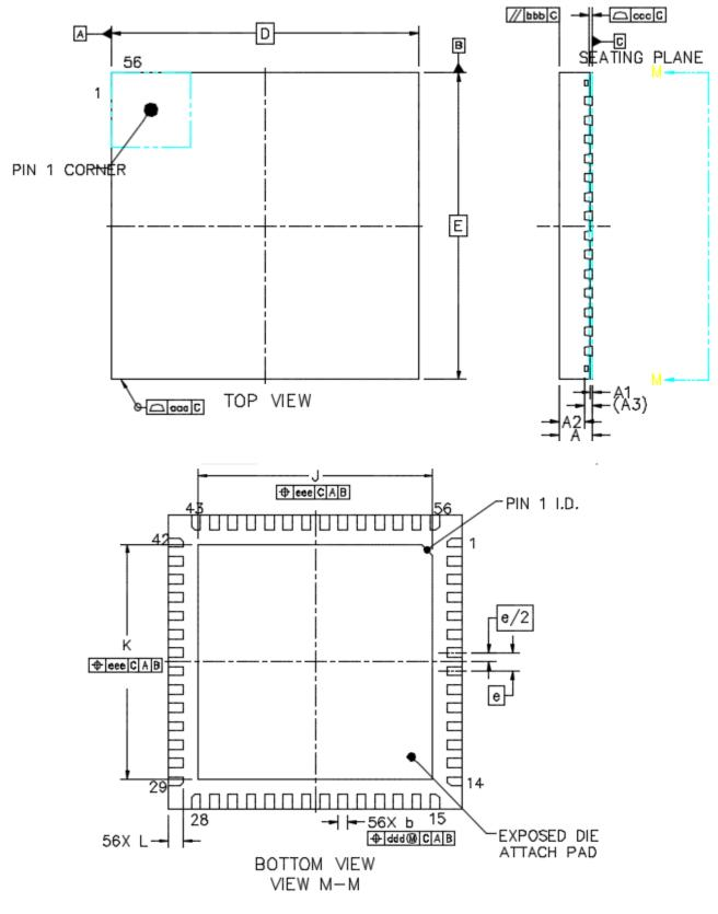
Figure 2.2. 56-Pin QFN
