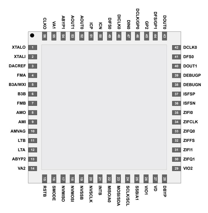
Figure 1.1. Si47961-62 Pinout Diagram
