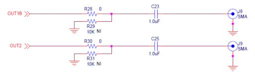
**Figure 5. Output Clock Termination Circuit**
