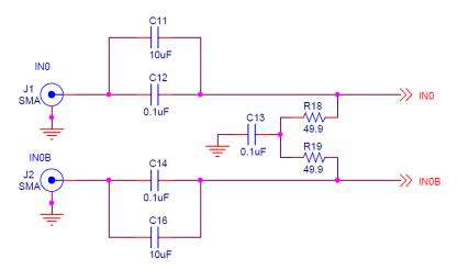
**Figure 4. Input Clock Termination Circuit**
