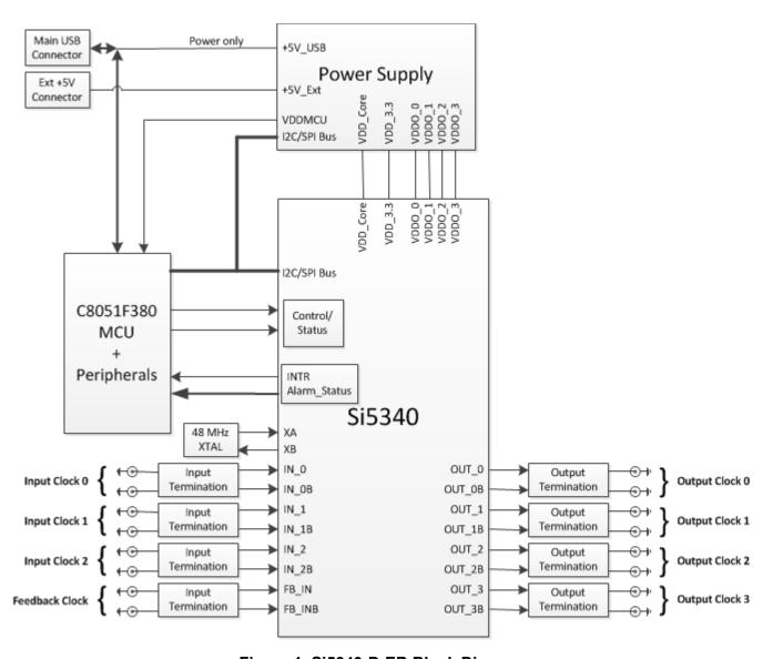
Figure 1. Si5340-D-EB Block Diagram
