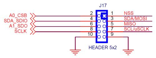
Figure 26. Serial Communications Header J17
