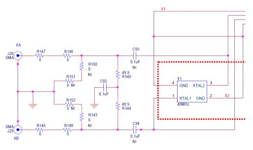
Figure 3. External Reference Input Circuit
